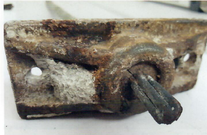
Fig. 20—Specimen No. 6: anchor, nonbearing front side.
