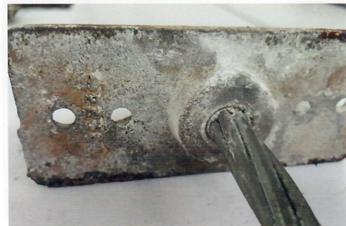
Fig. 21—Specimen No. 6: anchor, bearing side.
