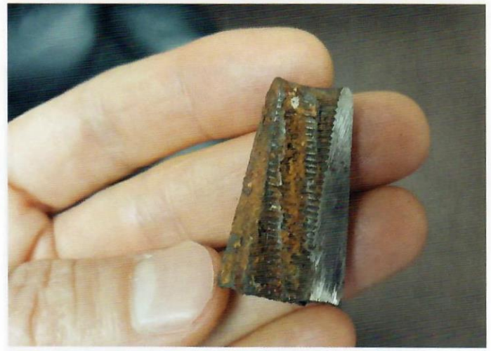
Fig. 7—Specimen No. 1: wedge serrated teeth
