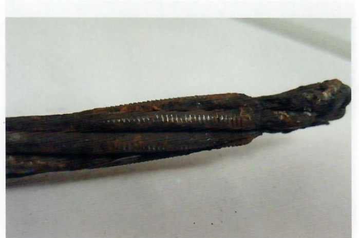
Fig. 8—Specimen No. 1: strand bite marks from wedge.
