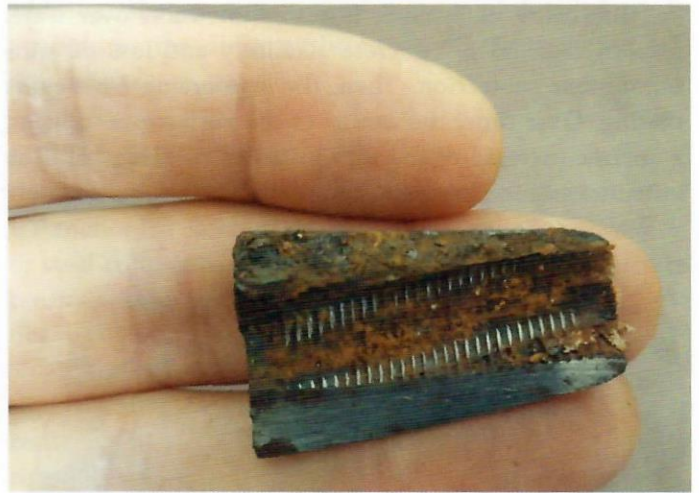
Fig. 6—Specimen No. 1: wedge serrated teeth.
