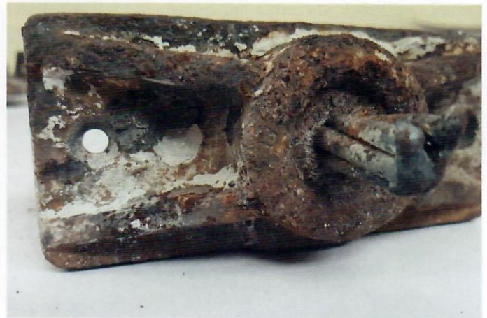
Fig. 16—Specimen No. 4: anchor, nonbearing side.
