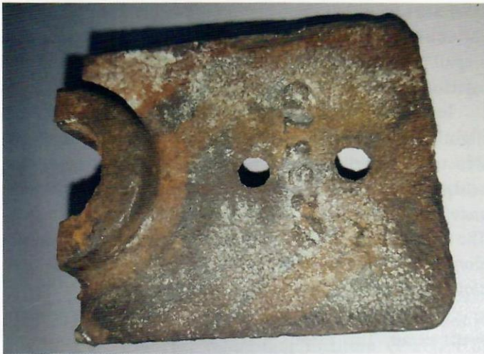
Fig. 3—Specimen No. 1: anchor, bearing side.
