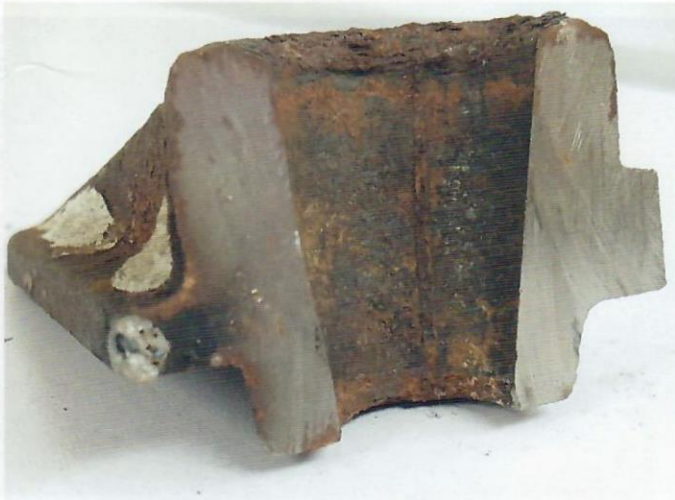
Fig. 4—Specimen No. 1: anchor cross section.
