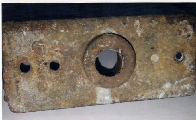
Fig. 10—Specimen No. 2: anchor, bearing side.
