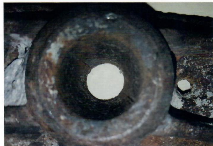
Fig. 13—Specimen No. 2: anchor, inside surface of wedge cavity.
