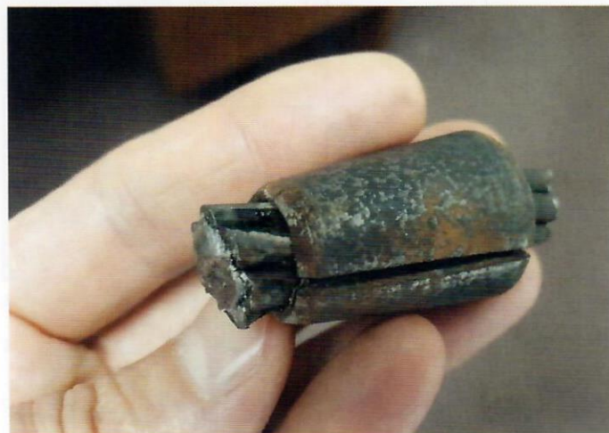
Fig. 11—Specimen No. 2: wedge and strand.
