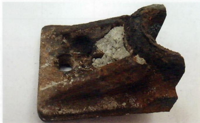
Fig. 2—Specimen No. 1: anchor, nonbearing front side.
