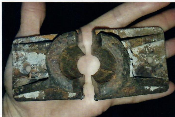
Fig. 1—Specimen No. 1: anchor, nonbearing front side.
