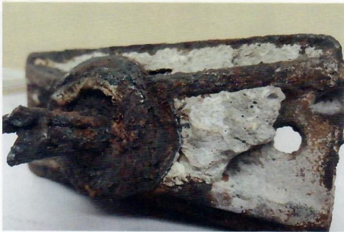
Fig. 14—Specimen No. 3: anchor, nonbearing side.
