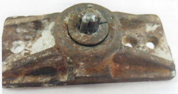
Fig. 9—Specimen No. 2: anchor, nonbearing side.
