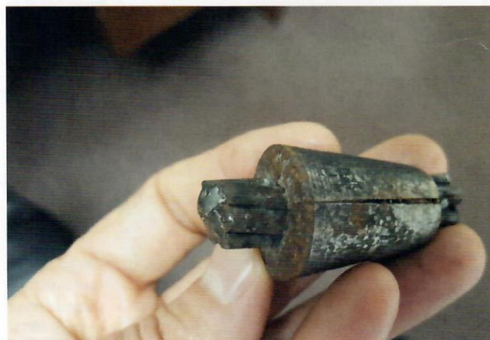
Fig. 12—Specimen No. 2: wedge and strand.
